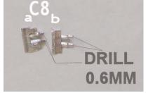
34.3) Fit the castings to the underside of the buffer beams centrally under each buffer as follows when looking end on: C8b left, C8a right. Remember you'll be working upside down so it's easy to get the order wrong! (See photo: MU Fittings.jpg)
