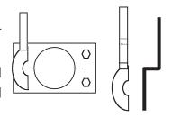
33) The buffer beams should be fitted directly to the floor molding. Take care as it is quite easy to glue everything together solid! With the floor in position, initially tack the buffer beam in place then remove the floor from the body and finish off the job, reinforcing the joint as appropriate. Remember the buffer beams will be holding the train together when in operation!
